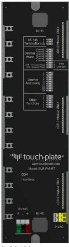
**Supported Baud Rates:** 9600, 19200, 38400 **8 Data Bits, Even Parity, 1 Stop Bit**
