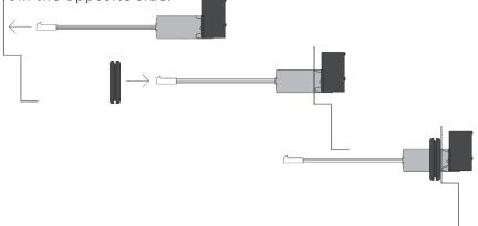
Relay Panels Post 2006: The relay mounting hardware (rubber grommet) is installed into the barrier strip by pinching it into the barrier strip and then the relay slides through the mounting hardware.
